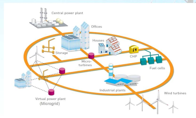
*Future:* Operation of system will be shared between *central and distributed generators*. Control of distributed generators could be aggregated to form microgrids or 'virtual' power plants to facilitate their integration both in the physical system and in the market.
